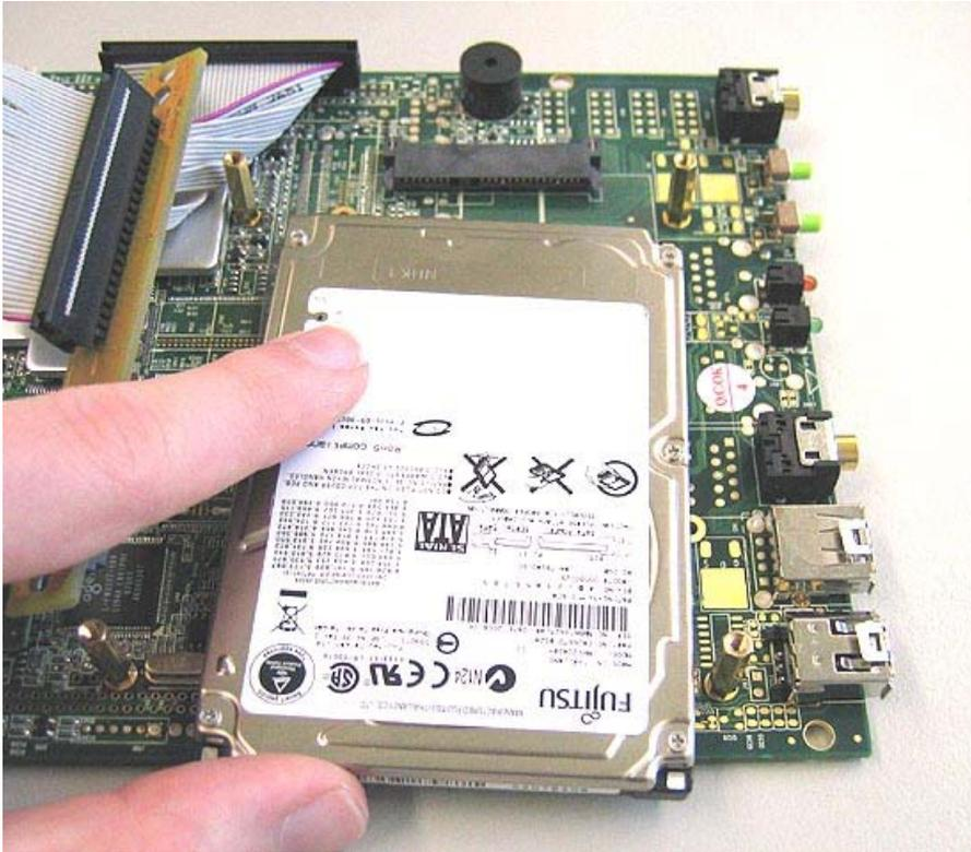
On the rear of the motherboard you can fasten the SATA HDD with 4 screws:
