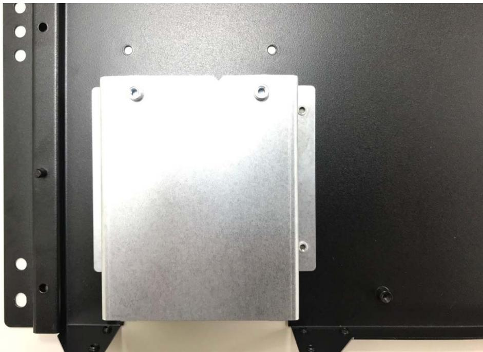
**Step 2.** Turn over the bottom cover and screw four screws as shown in the picture.
