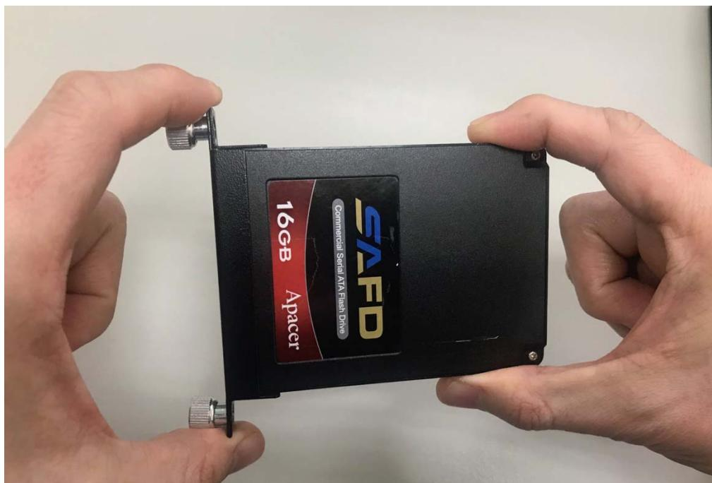
**Step 9.** Screw two screws on both side as shown in the picture.
