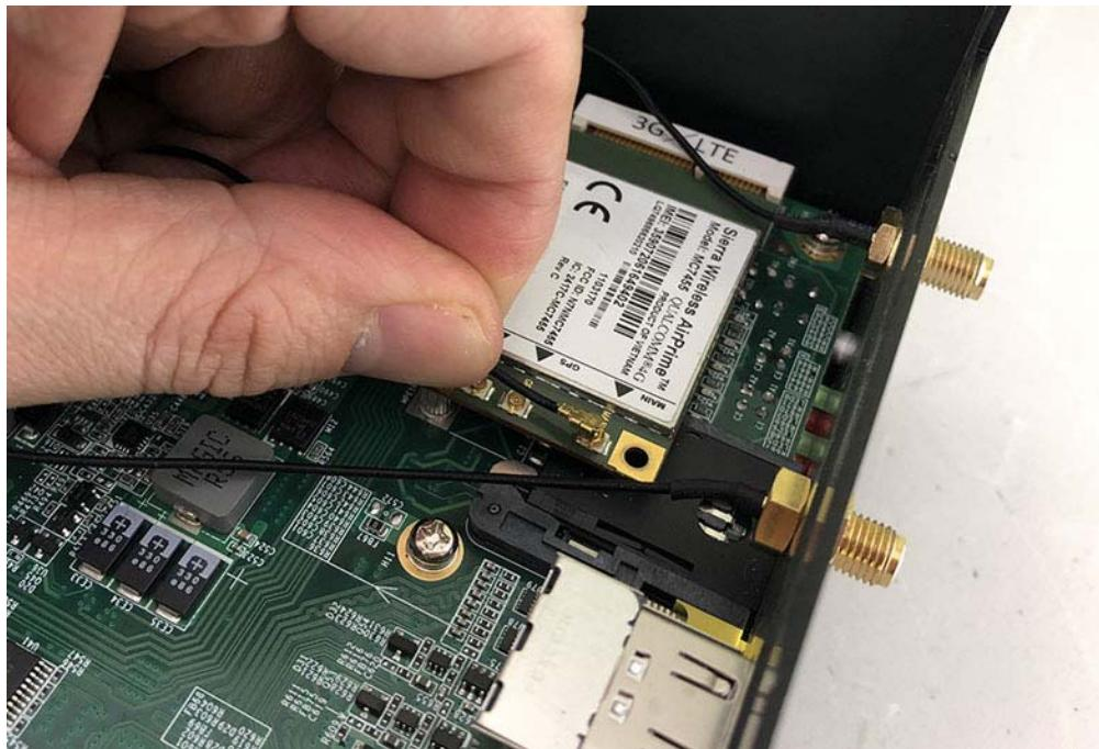
**Step 6.** Take the Ipxe Connector and press on the wifi module as shown in the picture.
