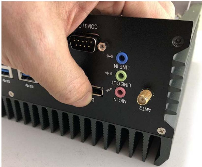
**Step 2.** Put the Washer into the SMA Connector as shown in the picture.
