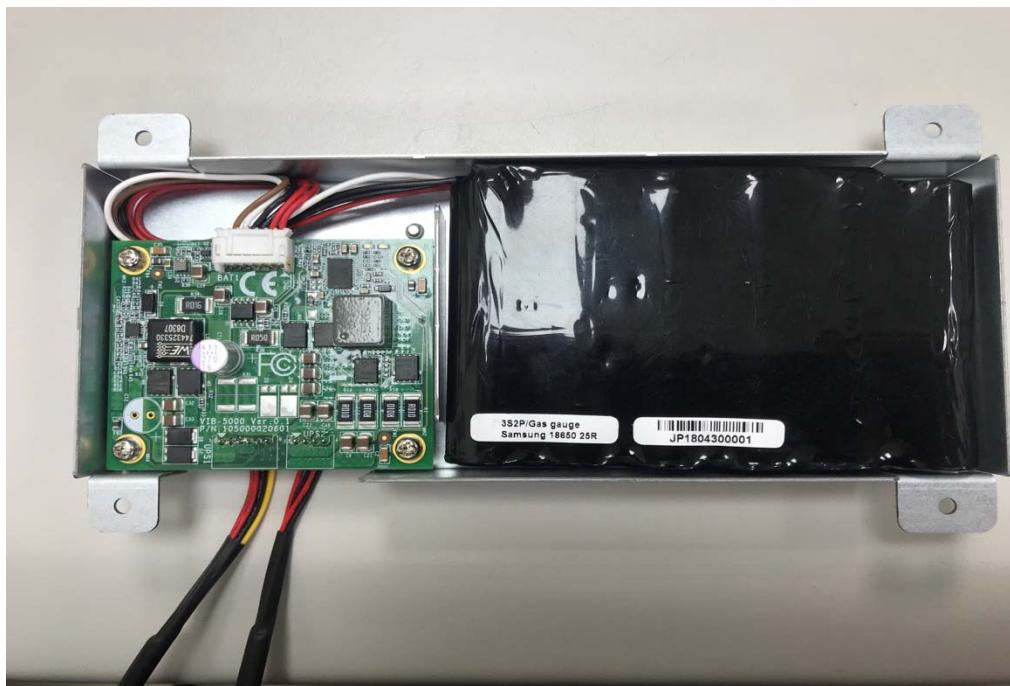
**Step 6.** Take the battery kit and screw four screws into the back cover as shown as picture.
