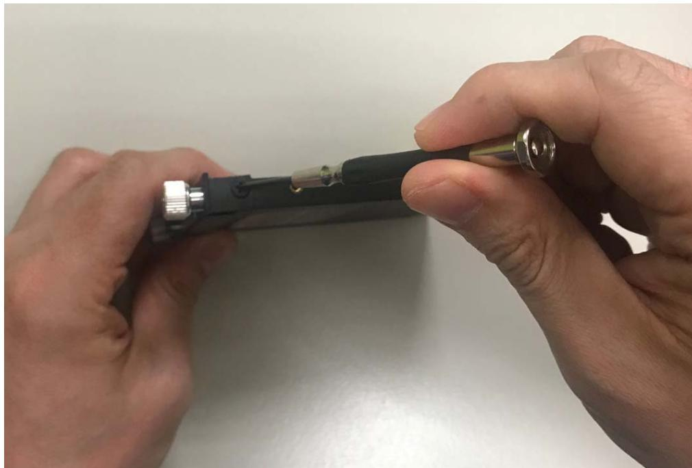
**Step 10.** Push the HDD Holder into the socket as shown in the picture.
