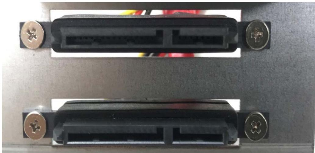
**Step 5.** Put SATA bracket and on the bottom cover and screw two screws as shown in the picture.
