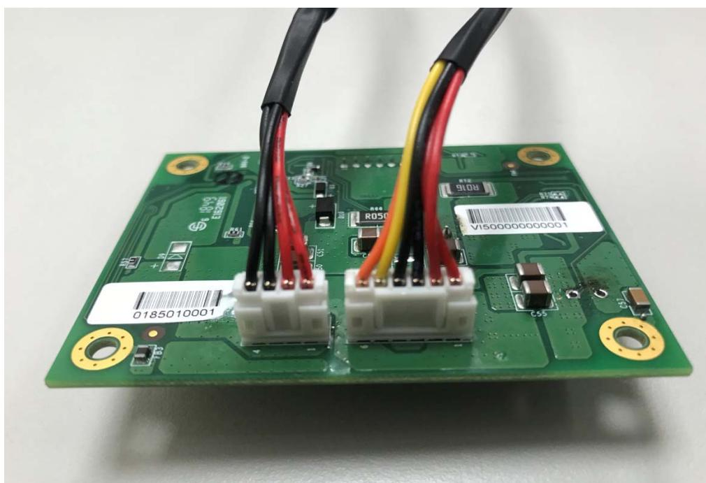
**Step 3.** Connect the battery with VIB-5000 on BAT-1 Socket.
