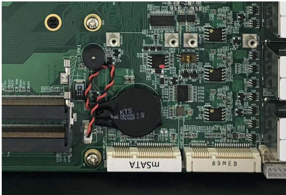
**Step 2.** Hold the Module with its notch aligned with the socket of the board and insert it at a 30 degree angle into the socket as shown in the picture.
