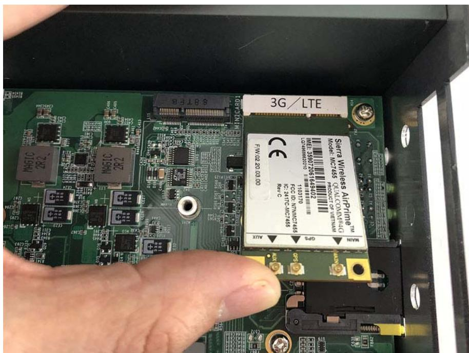
**Step 3.** Screw one screw to the holder as shown in the picture.
