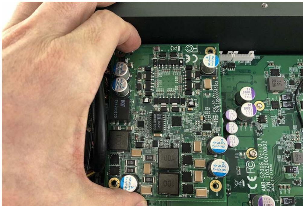
**Step 3.** Put the Heatsink on the POE module as shown in the picture
