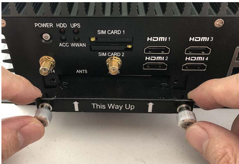
**Step 11.** Fully insert the HDD Holder into the socket until a “click” is heard as shown in the picture.
