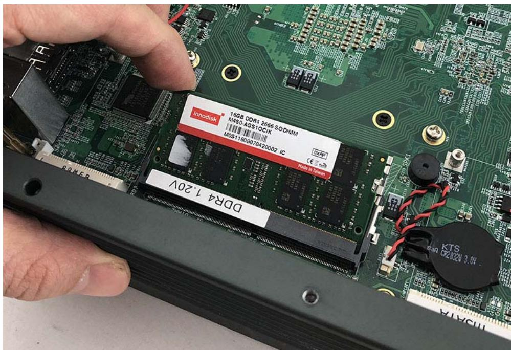
**Step3.** Press down on the Memory so that the tabs of the socket lock on both sides of the module as shown in the picture.
