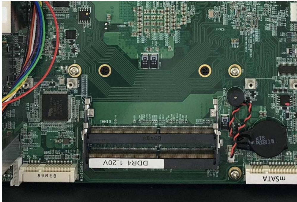
**Step2.** Hold the Memory with its notch aligned with the Memory socket of the board and insert it at a 30-degree angle into the socket as shown in the picture.
