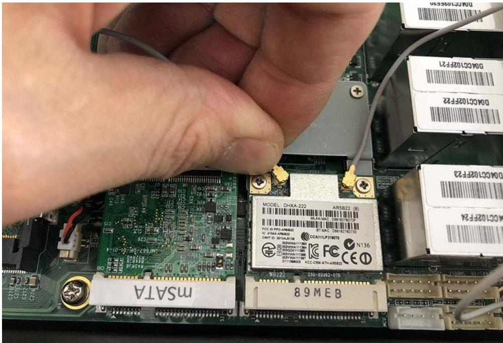
**Step 7.** Take the Ipex Connector and press on the GPS module as shown in the picture. (GPS)
