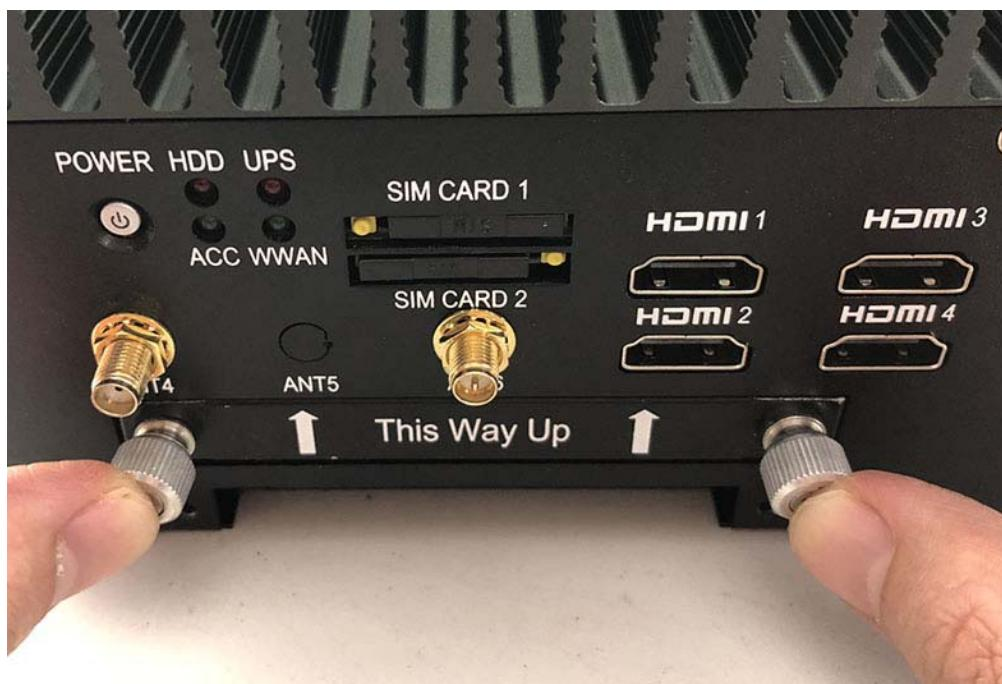
**Step 12.** Tighten to Storage Bracket screws as shown in the picture.
