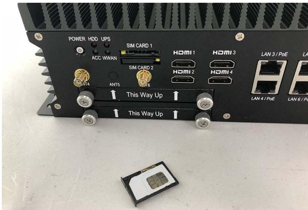
**Step 4.** Take the SIM card holder and Insert it into the socket as shown in the picture.
