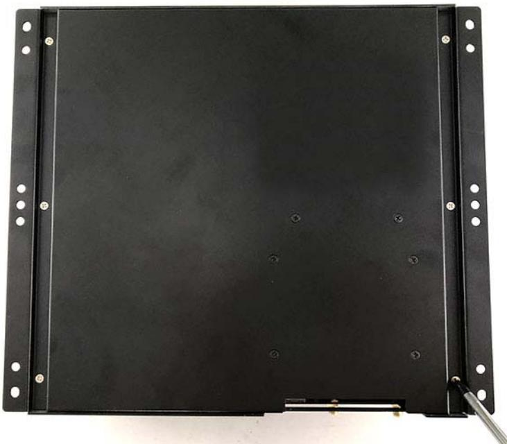
**Step2.** Unscrew the three screws of the Front Panel as shown in the picture.
