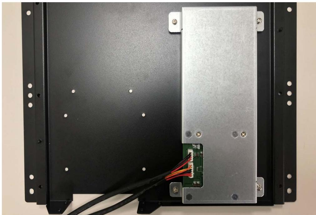
**Step 7.** Connect the battery kit with motherboard on UPS1(6pin) & UPS2(4pin) location as shown as picture.
