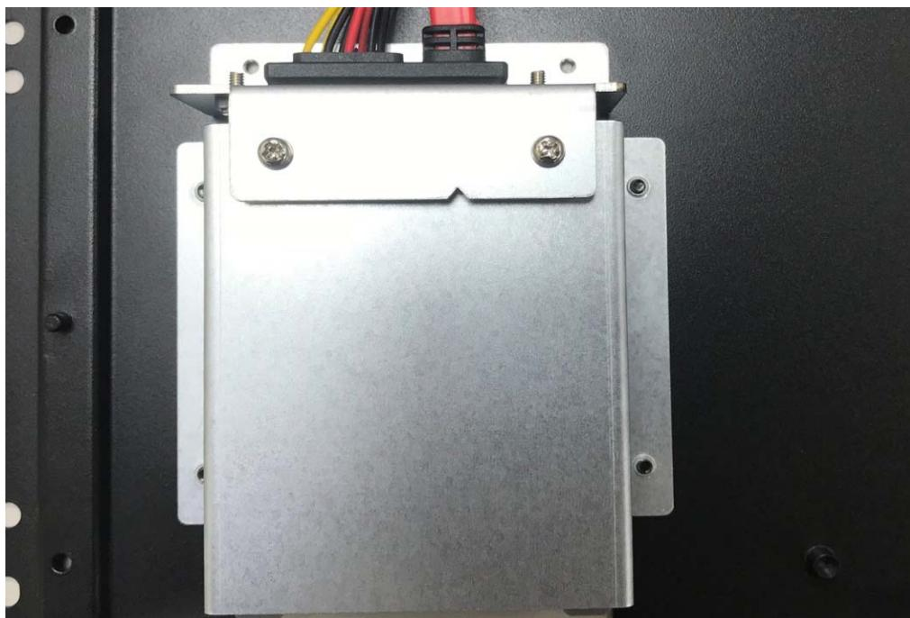
**Step 6.** Turn over the bottom cover and screw two screws as shown in the picture.
