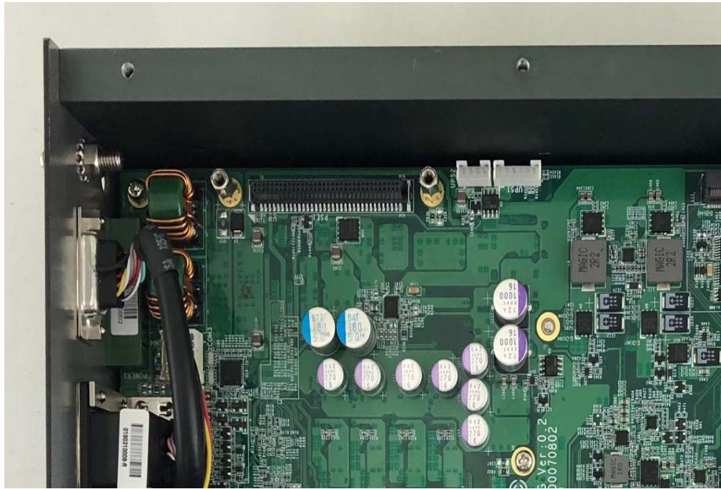
**Step 2.** Put the POE-8P module on the motherboard as shown in the picture
