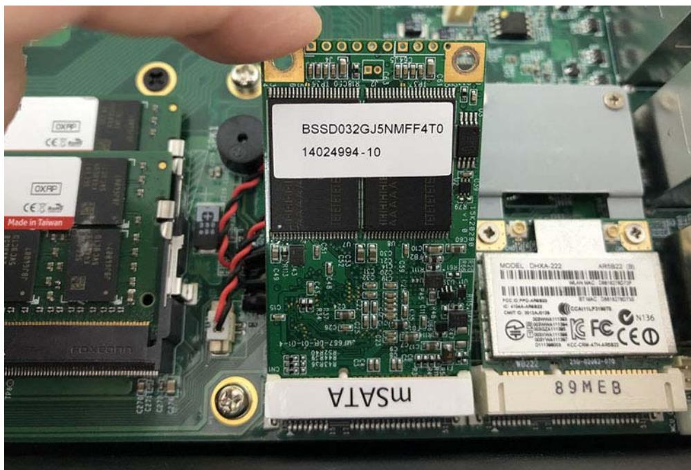
**Step 3.** Screw two screws to the holder as shown in the picture.
