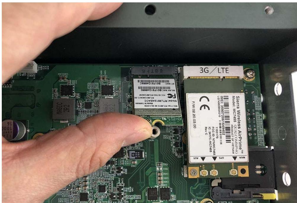
**Step 3.** Screw one screw to the holder as shown in the picture.
