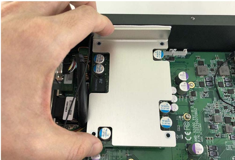
**Step 4.** Screw the four screws as shown in the picture
