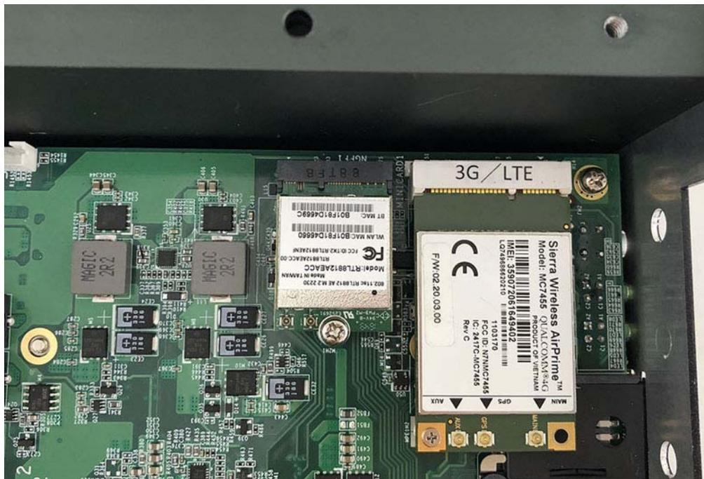
**Step 6.** Take the Ipxe Connector and press on the M.2 module as shown in the picture.
