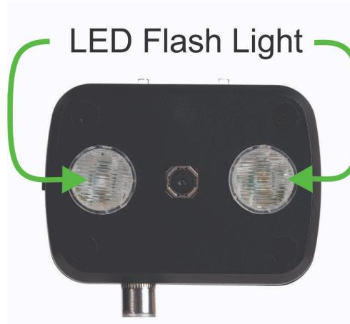
NORVI AI Optic has high-power LEDs designed to provide bright, white light with high efficiency. The Flash Lights are controlled via the IO Expander PCA9536DGKR. The communication with the IO Expander is done using the I2C protocol.
