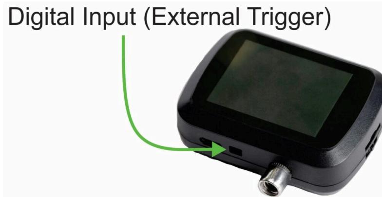
An external sensor can be connected to the digital input terminal and photos can be taken without having to use the internal trigger button.
