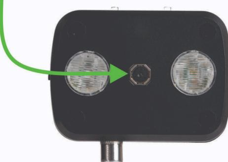
The OV5640-AF camera module includes an integrated auto-focus feature with a resolution of 5 megapixels.
